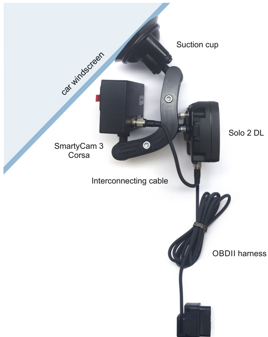
Pic 5: Cable connection on final layout
