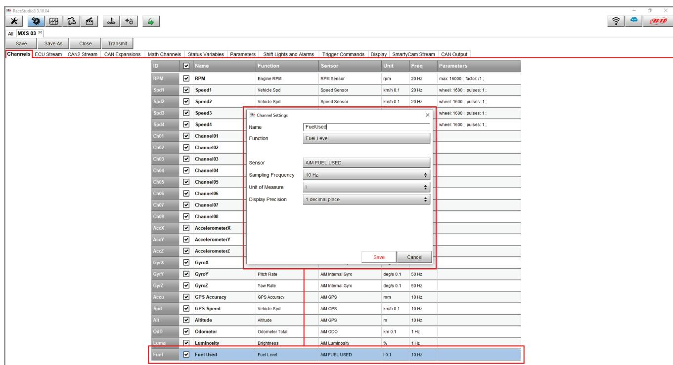
Once these first settings are done, click Save and they will be stored by the software, so that the Fuel Used channel can be utilised in the other device configuration section tabs.
