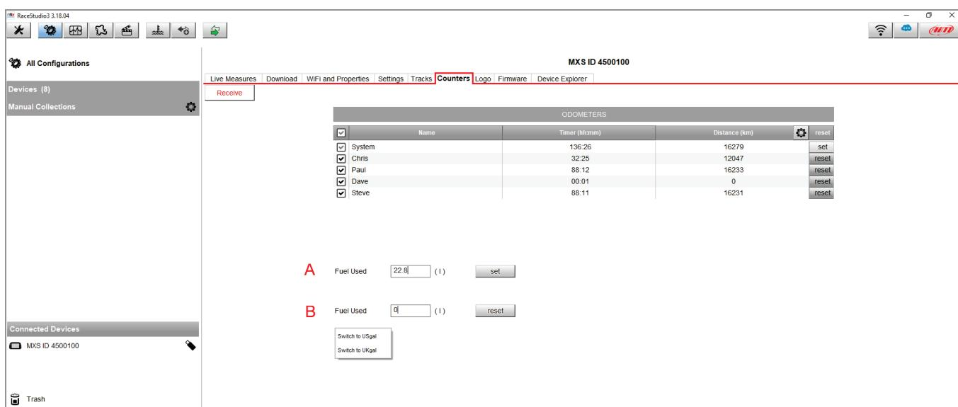
The used fuel quantity value can be reset from the devices too:
