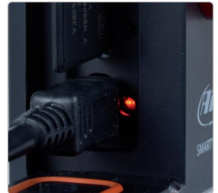
If SmartyCam HD is powered by an external 12V power source or by AiM CAN network a plug icon is shown on the display and the video recorder works in a fully automatic way switching ON/OFF with the external power. Meanwhile the internal battery too is charged and the bubble right of the plug changes its colour according to the battery charge level. When the battery is fully charged the bubble comes green.
