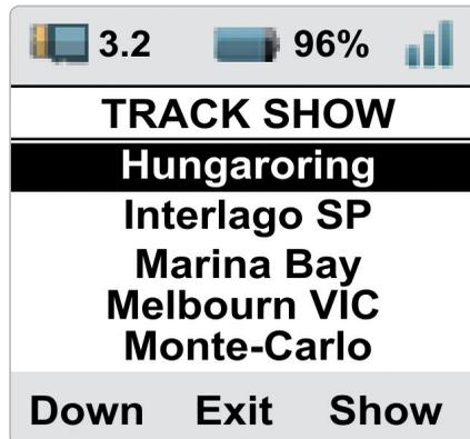
To switch to **MANUAL** mode press “Change” in Auto mode and “MANUAL SEL” enables. If a track has been selected it will be shown with the related distance from current position (Silverstone GP, 679 miles away in the left image below). To select another track press “Sel” and the list of all track loaded in your SmartyCam HD will be shown.
