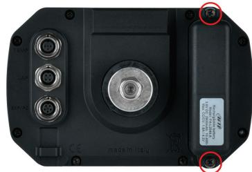
To recharge the battery remove it from the logger unscrewing the screws highlighted here above on the right, place it on the charger shown here below on the left. The charger has a green LED on the bottom (right image below) that blinks while charging the battery. When the battery is charged it becomes steady.
