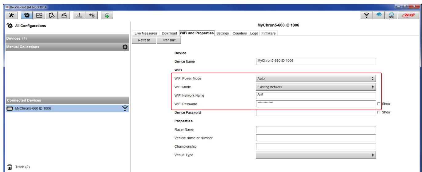
Here above you see a device “MyChron5 660 ID 1006” that is switching from AP to WLAN (“Existing Network”) mode.
