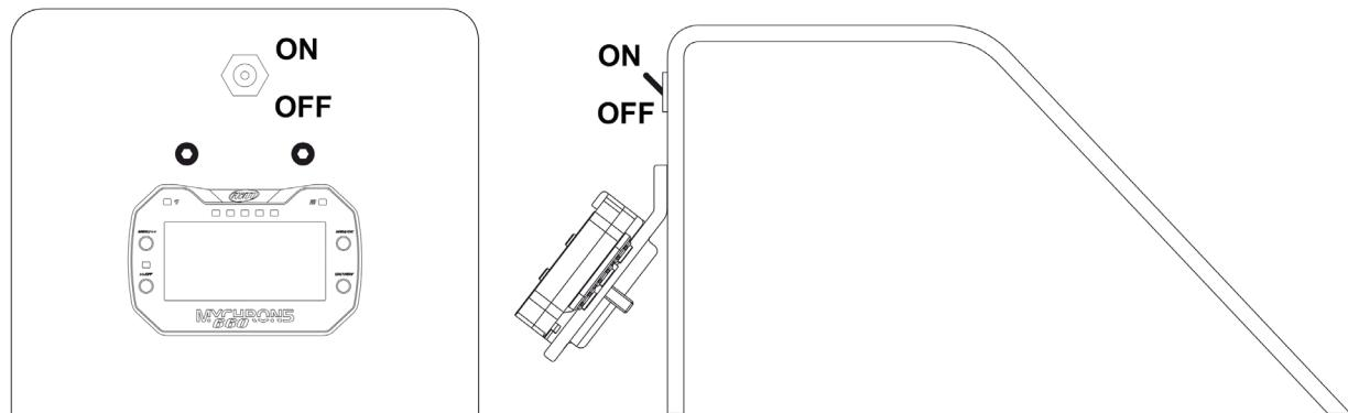
As shown here above on the right the logger needs a bracket. Use an aluminium or steel self-made bracket 0.1" (2.5 mm) thick so to resist the vibration when the engine is on. Firmly fix the bracket to the vertical bulkhead and then fix MyChron5 660 to the bracket. Please be careful not to overtighten the mounting nut; this can cause damage to the display unit case.
