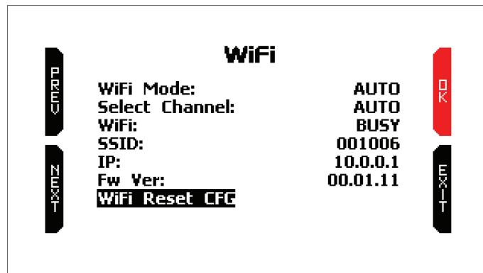
MyChron5 660 Wi-Fi working mode can only be changed using RaceStudio3 software. Two possible Wi-Fi modes are available:
