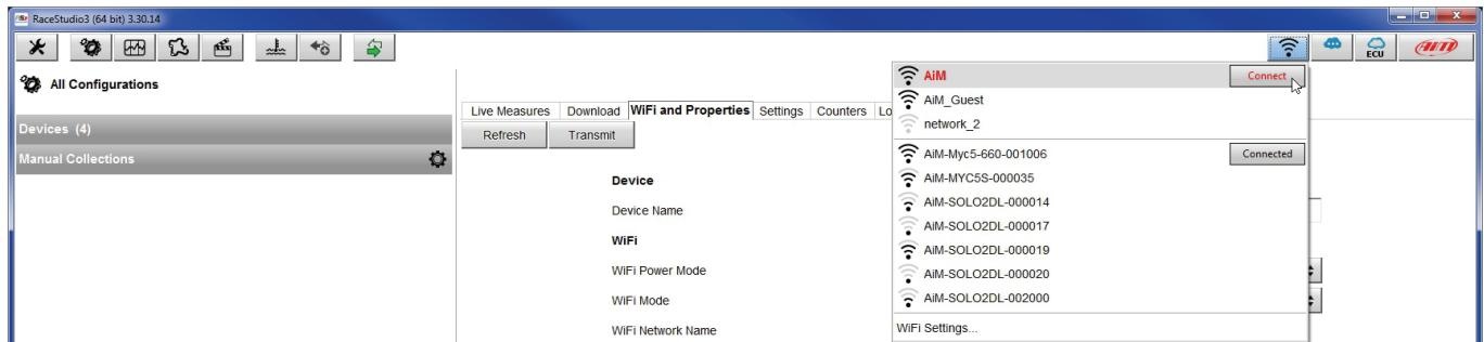
When the PC is authenticated to the network called "AiM" it can see all devices you configured to access the same network. In the image below three AiM devices are connected to the same "AiM" WLAN.
