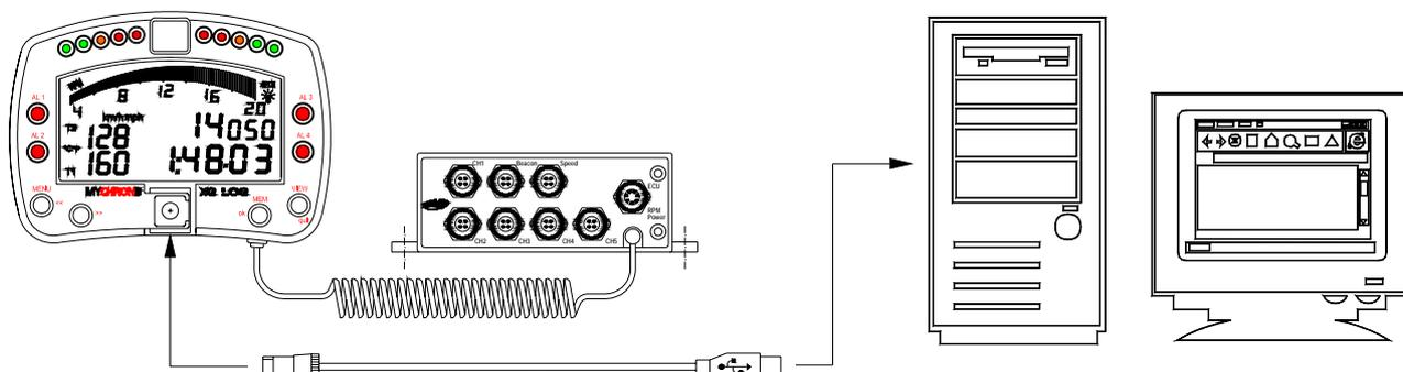
Figure 6: How to connect Your **MyChron 3 XG LOG** to the Pc
