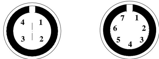
4 & 7 pins female Binder 712 connectors pinout: external view
