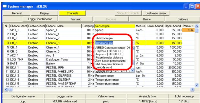
To set an input channel, double-click on the cell corresponding to the desired one: the pop up window circled above appears.
