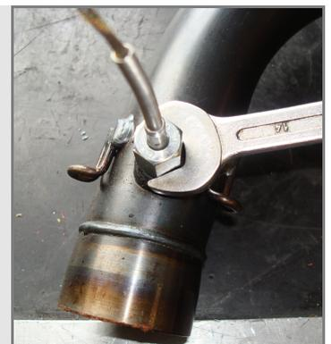
**Warning:** when running the thermocouple cable along the chassis keep it as far as possible from other cables (like RPM cable or receiver one) to minimize possible interferences.
