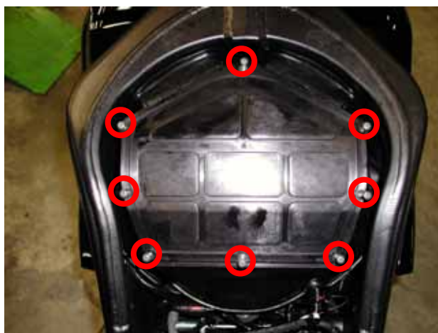
Figure 20: Location of the Airbox screws.
