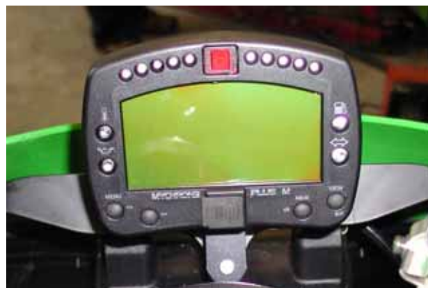
Figure 10: MyChron 3 Plus correctly installed.
