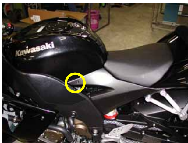
Figure 14: the screw that fixes the plastic fairing to the bike chassis
