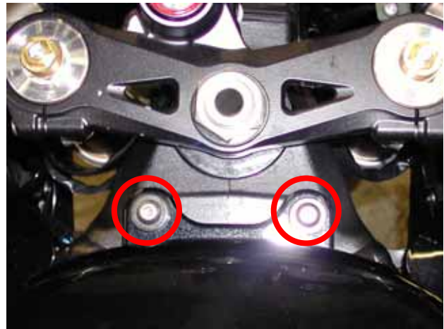
Figure 16 these screws have to be removed
