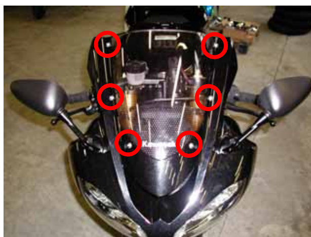
Figure 1: front transparent fairing – screws location
