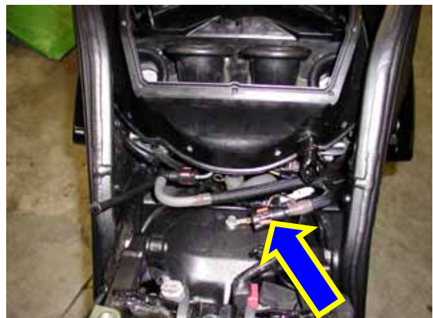
Figure 18: the hose that takes the fuel to the engine
