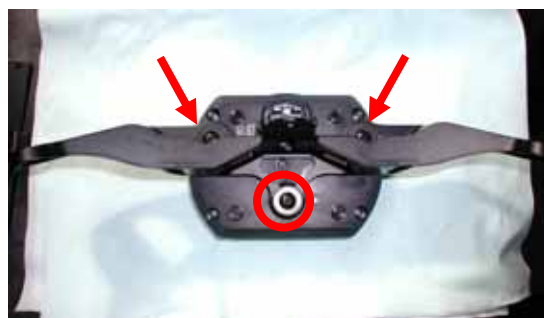
Figure 6: screws that fixes the stock dash
