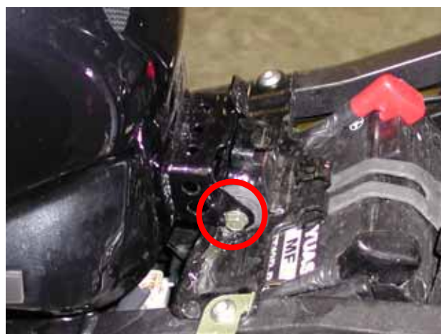
Figure 15: one of the screws that fix the gas tank.
