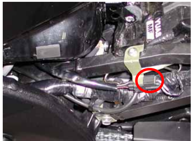
Figure 17: this black connector has to be removed
