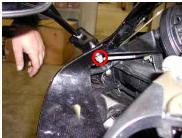
Figure 2: .internal screw to remove.
