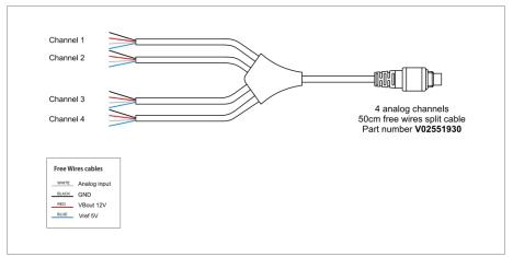
Harness for 2 thermocouples and two AiM sensors.
