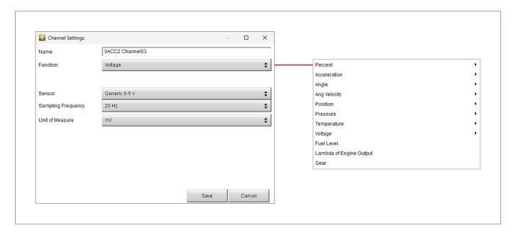
When the configuration is finished save and transmit it to the logger (MXG 1 in the example) using the software top left keyboard.
