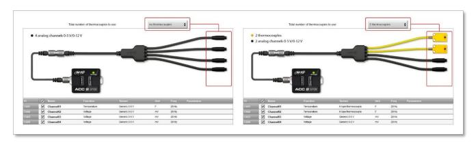
ACC2 supports up to four K type thermocouples. Once the number of thermocouple(s) to be connected is fixed the software warns you and the corresponding channel(s) switches to "Temperature".
