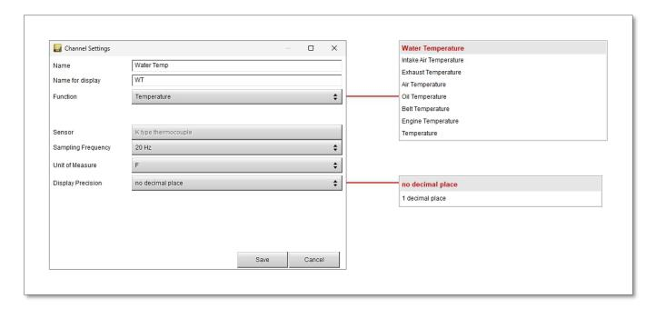
In the similar way you have to configure the remaining channels: click the channel to set and a setting panel is prompted; a lot of possible function can be set according to the kind of sensor you connect to ACC2.
