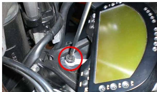
Figure 8: fixing the front screw.
