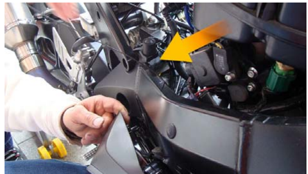
Figure 15: ground cable runs along the bike chassis.
