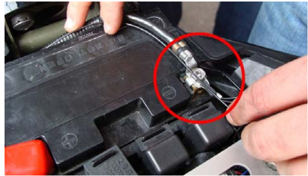
Figure 16: connection of ground cable to the battery negative pole.
