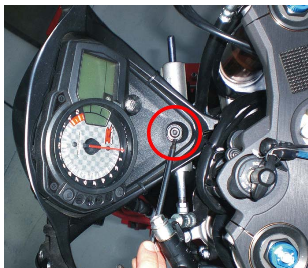
Figure 2: front fixing bolt of the stock dash.
