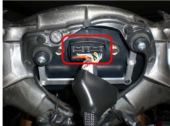
Figure 10 : MXL wiring connection.
