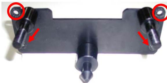
Figure 7: Anchor plugs are fixed to the bracket
