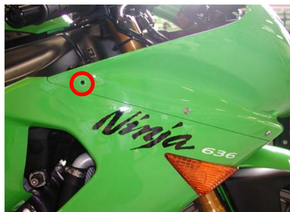
Figure 2: .Lateral screw to remove.
