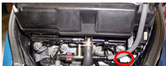
Figure 15: the gas tank has been uplifted
