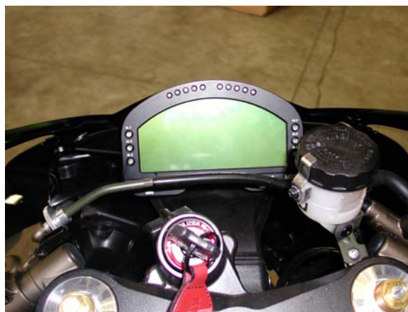
Figure 10: MXL correctly installed.
