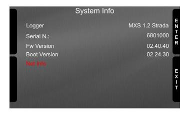
"Net info" option appears only if an expansion is connected to MX Strada, GPS included and pressing "ENTER" button the information of these expansion are shown as below.
