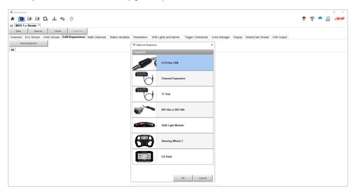
Select the CAN expansion to set and press "OK". Each expansion needs to be set filling in the related panel.
