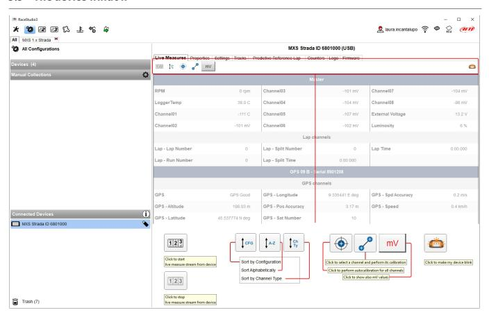
Clicking the device, bottom left of the software page, the software enters device page. Top of the view are six buttons, some of whose change its function pressing it as explained in the above image.
