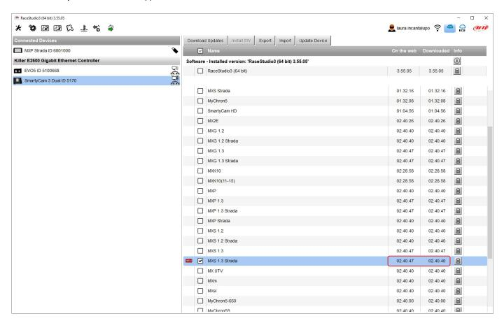
Once the new firmware has been downloaded connect your device to the PC using the USB cable to perform a firmware upgrade. In a few seconds the device is ready.
