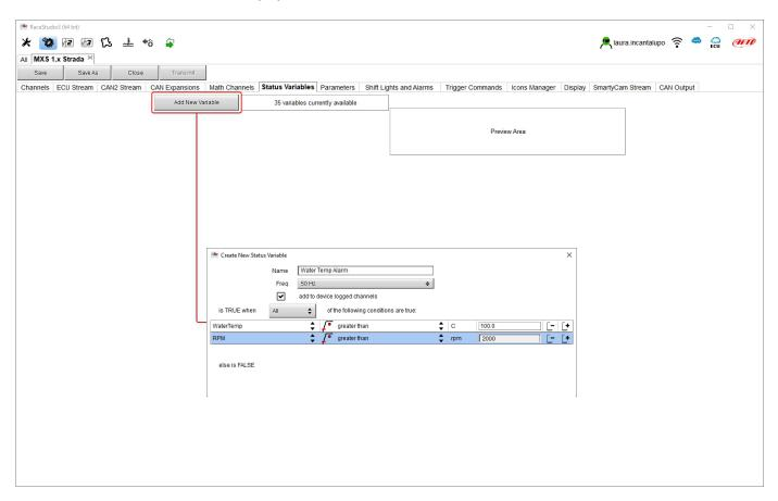
The Status variables can be used as any other channel, so they may be seen online, transmitted to the CAN stream, recorded, used for triggering a command or for turning ON a LED or an Icon.
