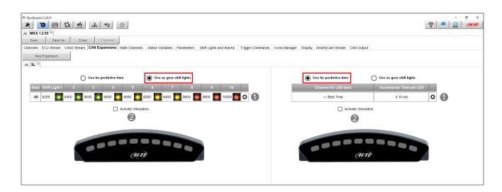
For both functions, clicking the gear button (1 - previous image), it is possible to set LEDs switching on strategies. For shift light function, the RPM threshold values can be set that, if exceeded, cause the LEDs switching on, each LED colour, reference channel and their switching on sequence mode (one at a time or all turned on till gear shifting).
