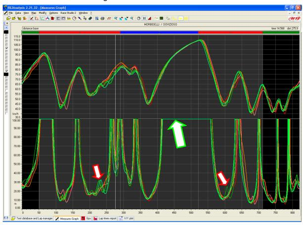
Bending radius increases on straights until very big values (green arrow in the figure); this is due to the fact that on a math channel point of view a straight is a corner with "infinite" radius and thereby very big.
