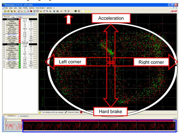
The graph shows there are not big differences between the two pilots, except for right corner entrances (area highlighted in red in the figure) where Morbidelli can better exploit the vehicle grip. To say the truth the difference with Dovizioso is really minimal.
